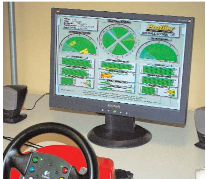
Before progressing to Level 2, students must complete a 1.5 hour session on the Profiler, which is designed to measure a driver's decisions-making skills, reaction time and field of vision.
